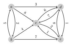
Find the weight of the shortest path from a to all nodes in the graph using Dijkstra's algorithm. Complete the table that indicates intermediate values of the upper bound  ${\tt d}$  of the distance from a after each iteration of the while loop. Fill in the column heading with the node that is considered at each iteration. Show your work by including the contents of the priority queue.
